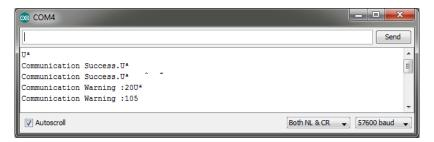
The Arduino responds with Communication warning 105. Warnings with a code of 100+ are issued by Arduino itself. You can see what this means by referring to the library header file:
