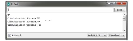
Communication warning 20 -> 0x14 in hex format. You can see what exactly this means in the error code reference section of the Supermodified datasheet:
