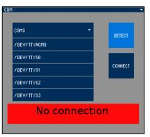
Then select your Arduino COM and click connect. If the message below the buttons says "Connection was successful" and the red color becomes green, the connection between the computer and the Arduino has been successfully installed.
