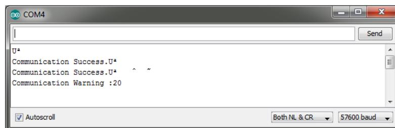
Communication warning 20 -> 0x14 in hex format. You can see what exactly this means in the error code reference section of the Supermodified datasheet:
